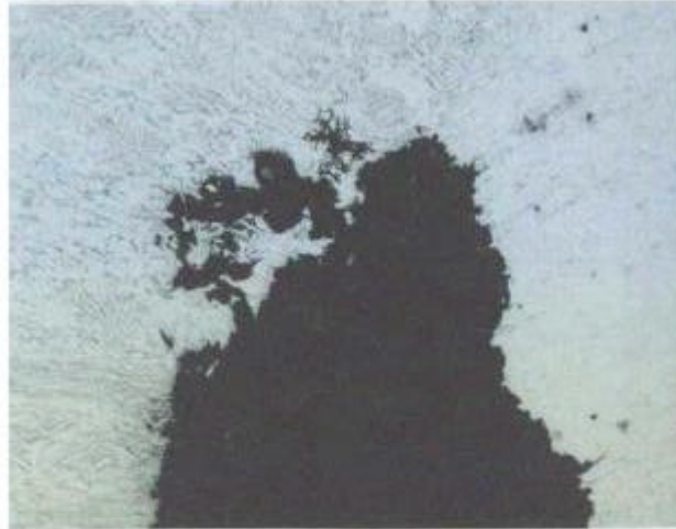
Figure 3—MIC-induced pitting in the weld region of a 304L stainless steel piping system.
