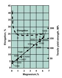
Comparison of yield strength & elongation with magnesium content for commercial alloys – annealed temper.
