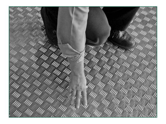
Welding: Aluminium treadplate can easily be welded with 5356 filler wire
