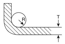
Sheet and plate are capable of being bent cold through an angle of 90 deg. around a pin having a radius equal to N times the thickness of the sheet without cracking.
