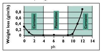
The corrosion resistance of aluminium alloys relies on a protective surface oxide film, which when damaged is readily repaired by the rapid reaction between aluminium and oxygen. However, the high reactivity of the base metal can give rapid corrosion if the film cannot be repaired, so aluminium alloys are not suitable for use with reducing media. Alloy 1100 can be anodised to improve the corrosion resistance by thickening the protective surface film.
